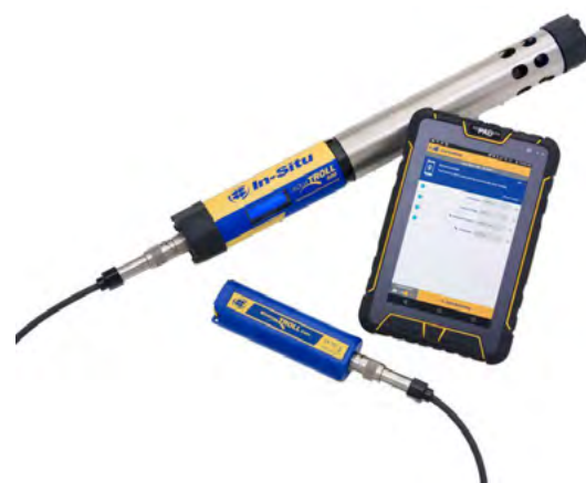
Figure 3.3 Aqua TROLL 500 Multiparameter Sonde and Wireless TROLL Com
