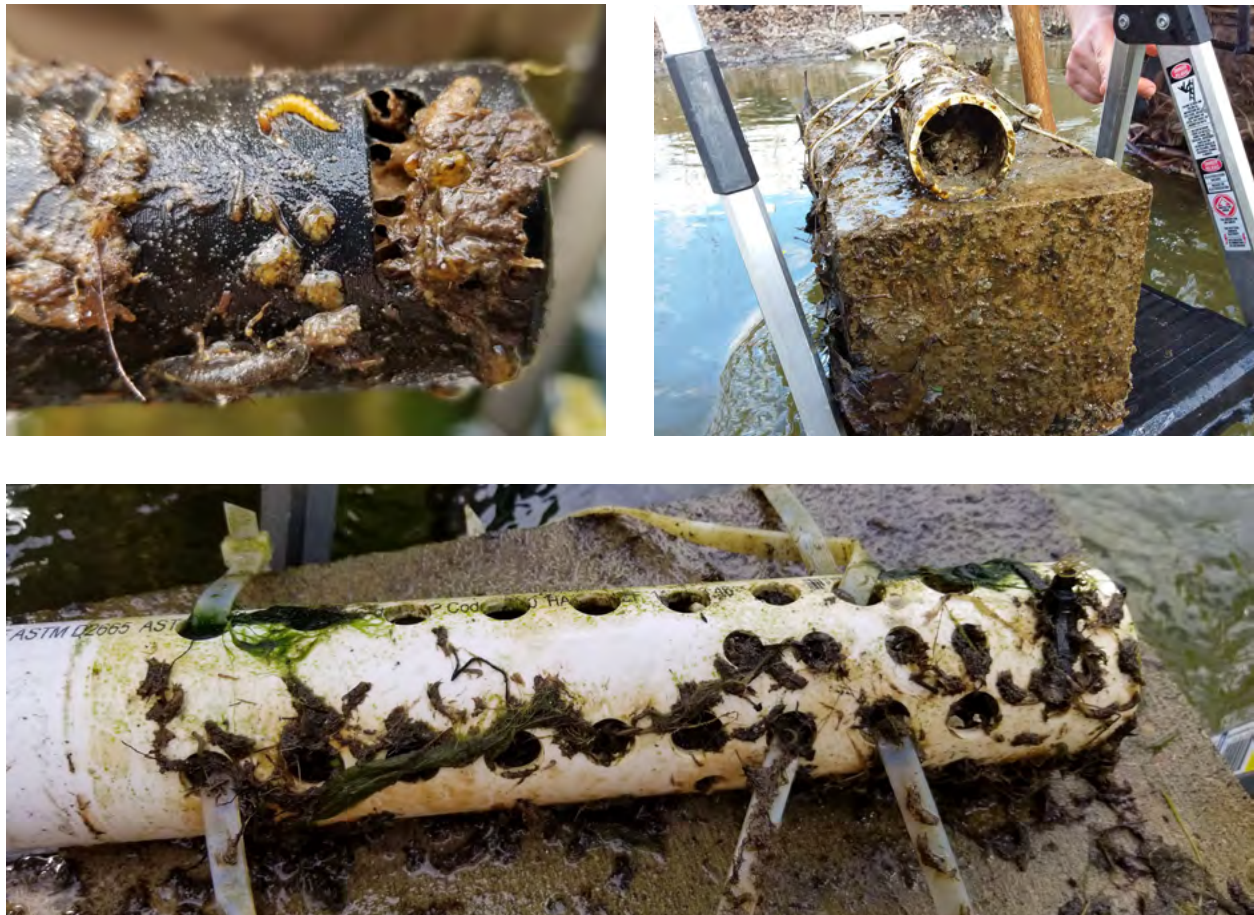
Figure 3.9 Examples of Fouling Observed on CTD-10 Sensors
