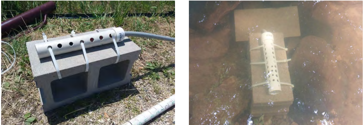
Figure 3.4 CTD-10 Sensor and Housing Assembly
