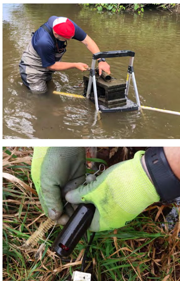
Figure 3.8 CTD-10 Sensor Cleaning and Maintenance
