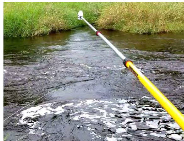
Figure 3.11 Assisted Sampler for Safe Sample Collection
