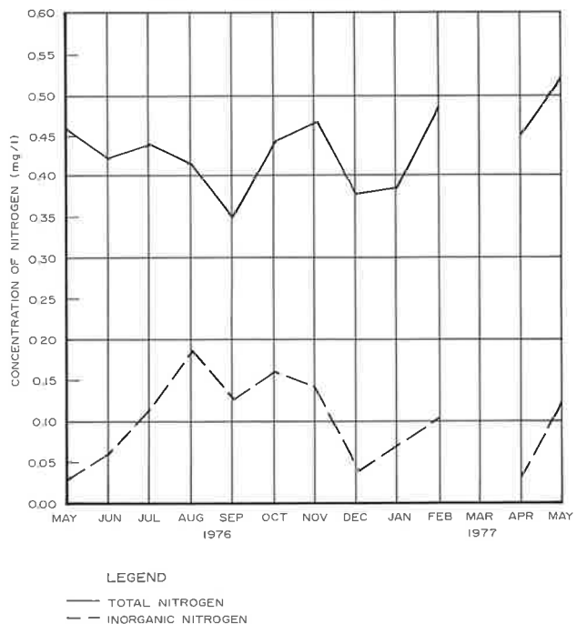
AVERAGE CONCENTRATION FOR ALL DEPTHS OF INORGANIC AND TOTAL NITROGEN IN FONTANA BAY: MAY 1976-MAY 1977
