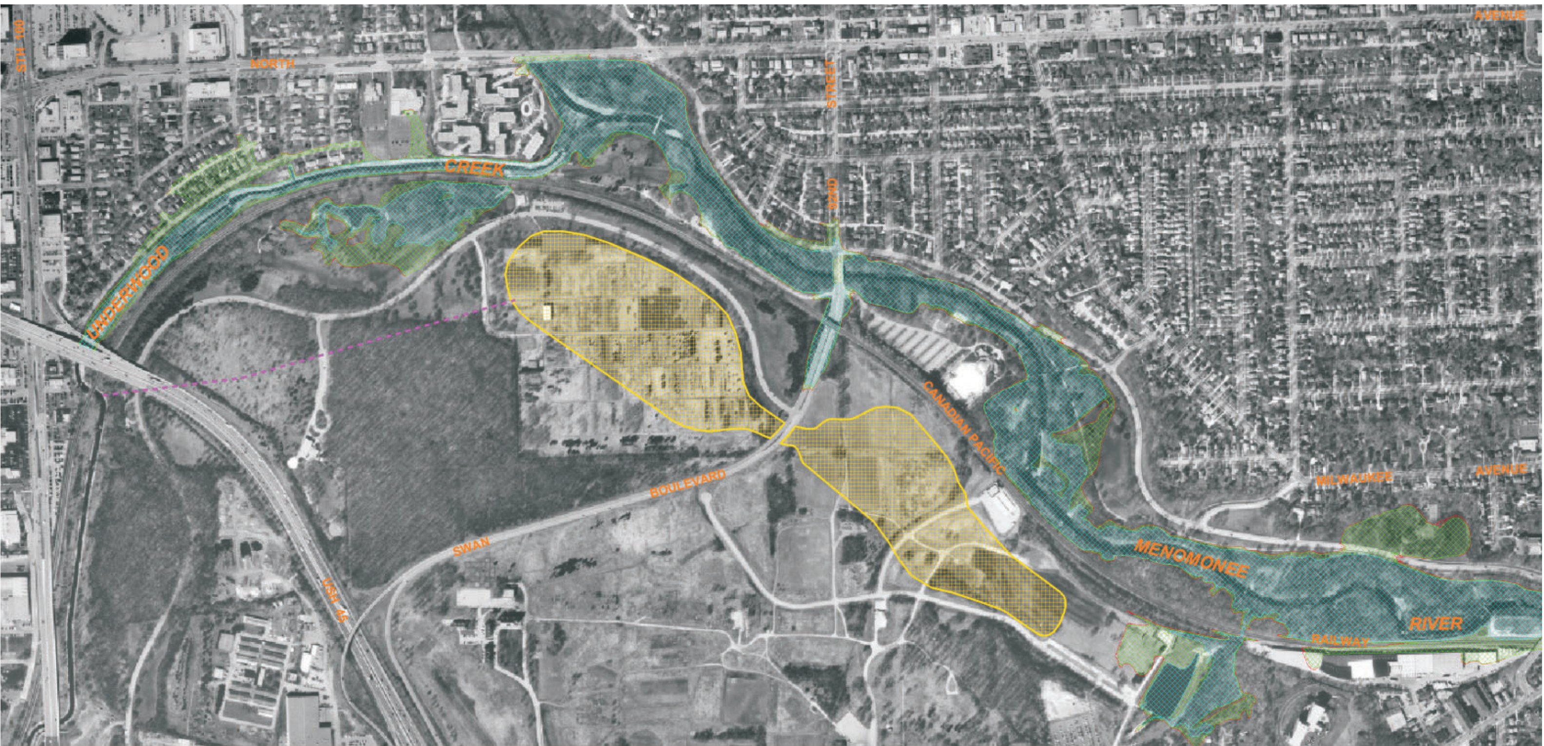
Map 2A Review of Proposed Milwaukee County Grounds Detention Basin Comparison of 100 - Year Floodplain Limits Planned Year 2020 Land Use Conditions
